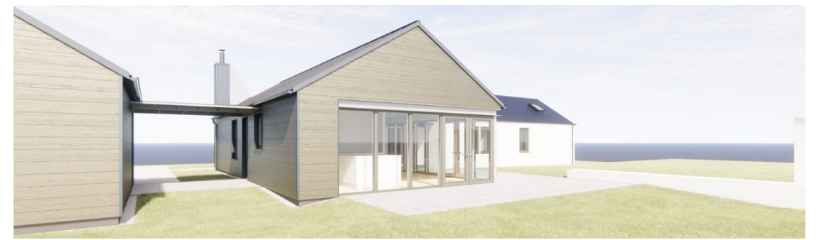
ABOVE - proposed image of cottage extension showing pitched roof with height and angle to match existing cottage and covered link between house and new garage
